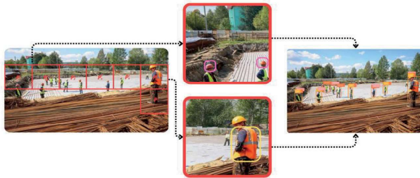
Figure 1. Scheme of operation of the Slicing Aided Hyper Inference (SAHI) method for detecting personal protective equipment at a construction site
