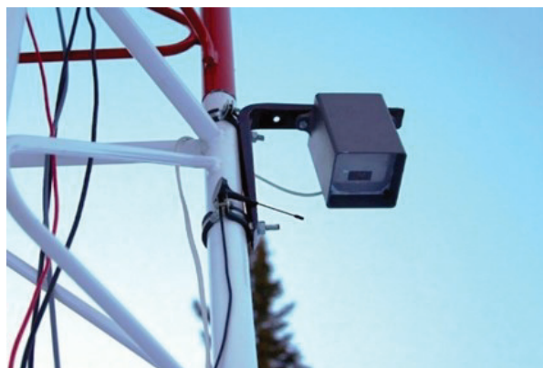
Figure 7. Receiver of data from a snow-temperature measuring rail.
