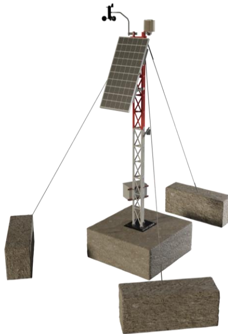
Figure 3. The type of construction of the snow avalanche base station.
