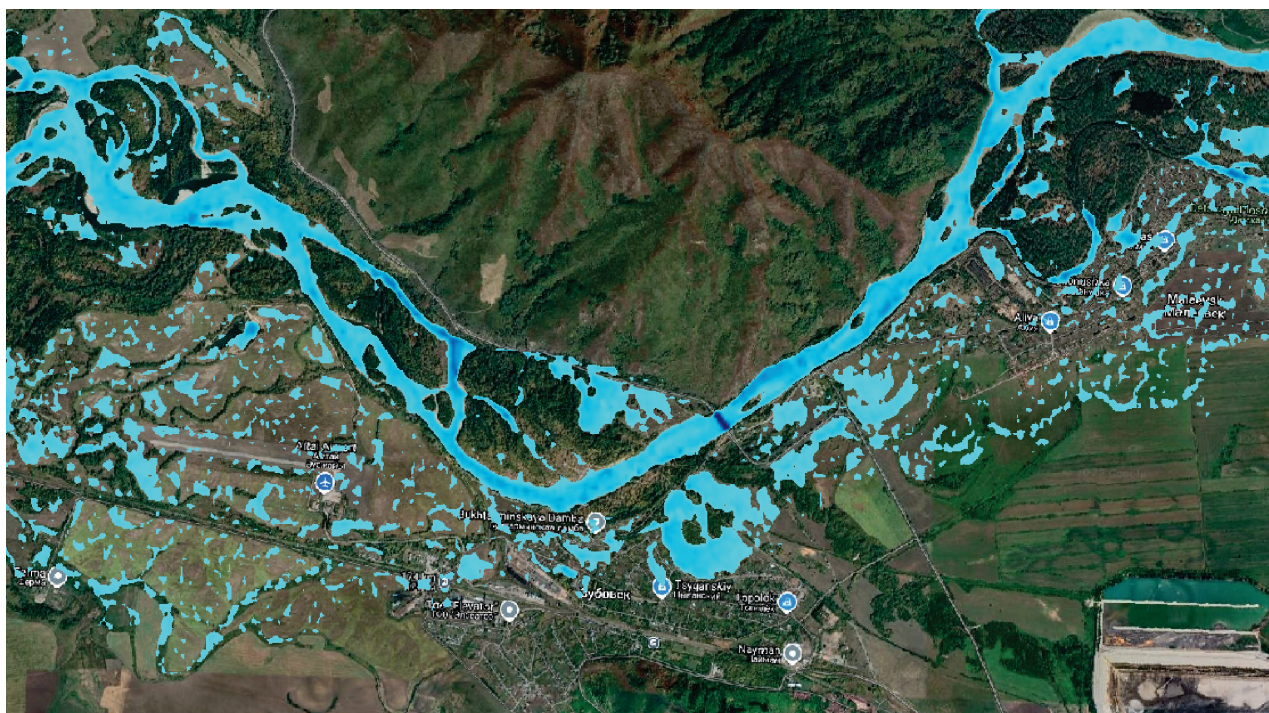
Figure 9. Flood map based on HEC-RAS 6.6 modeling results. Blue shades correspond to different flood depths.
