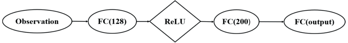
Figure 2. Actor network structure of the DDPG: FC(128) - fully connected layer with 128 neurons; FC(200) – fully connected layer with 200 neurons; FC(output) – fully connected layer that produces an output
